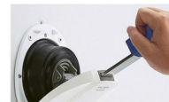
BILGE PUMP OSR reference 3.23.1 c) e) Bilge pump, manual, permanently installed, operable with all cockpit seats. Removable bilge pumps handle retained by lanyard.
