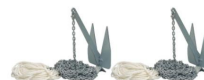
ANCHORS OSR reference 4.06.1 Two unmodified anchors with suitable combination of chain and rope, ready for immediate assembly, and ready for deployment within 5 minutes, except for boat less than 8.5m LH there shall be 1 anchor meeting the same criteria.
